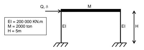
a) Calculate the frequency of vibration of the system.
